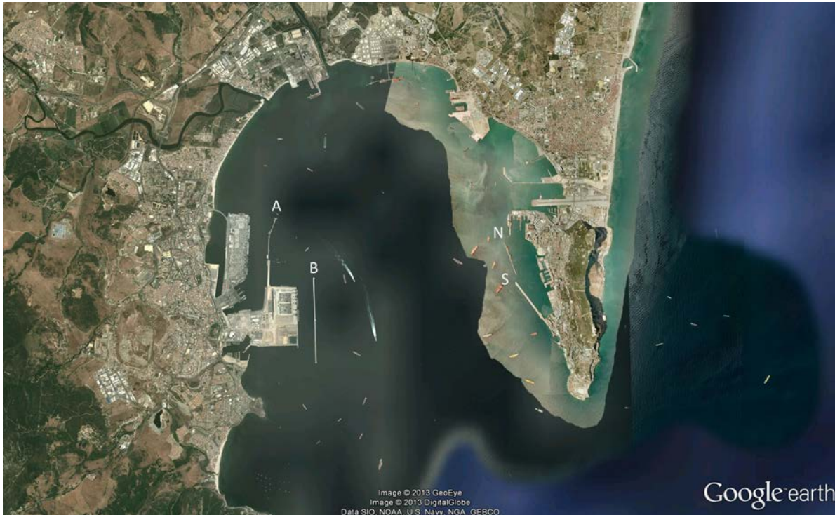
Figure 9 Gibraltar Bay showing breakwaters at Algeciras, with vertical wall frontage (A) and wave screen frontage (B) and Northern (N) and Southern (S) entrances to Gibraltar Harbour
