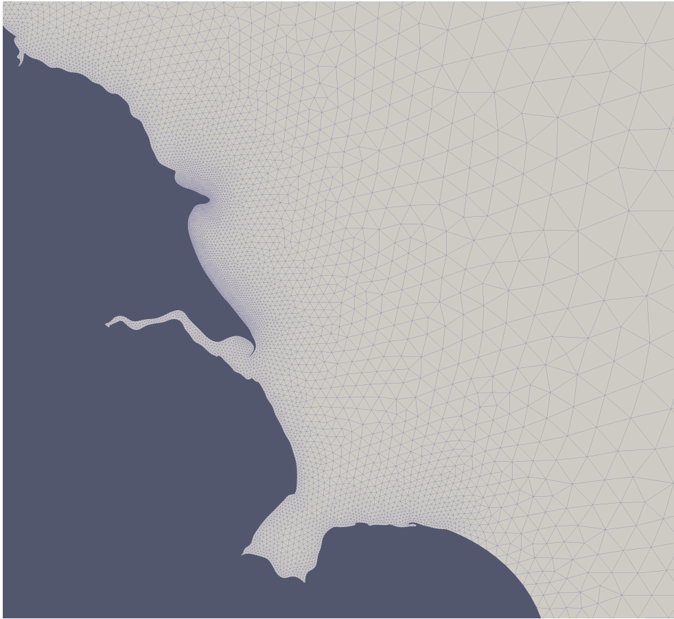
Figure 3.13: A zoom-in of the mesh for the European continental shelf tidal model, showing details of the finer mesh around the hypothetical outfall site.
