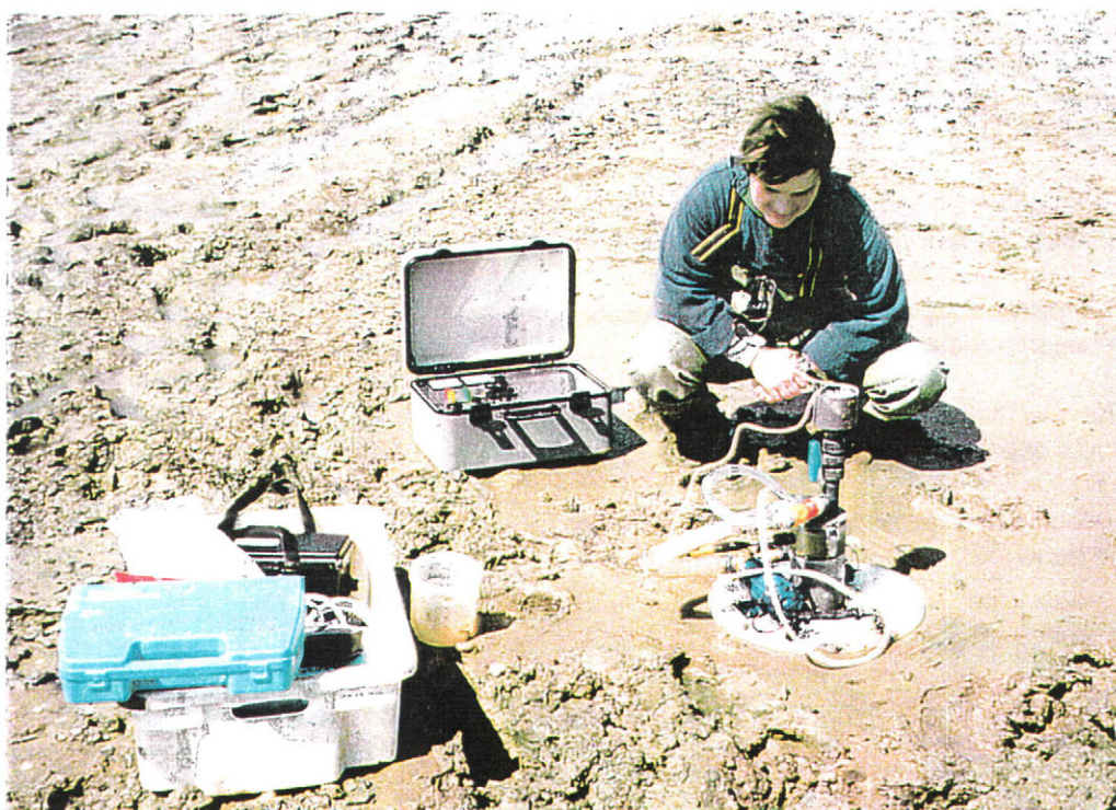
Plate 2 SedErode in action at West Mersea during testing
