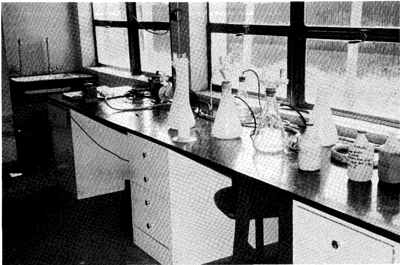
Plate 3 Water Quality and Pollution Control Centre vacuum filtration equipment
