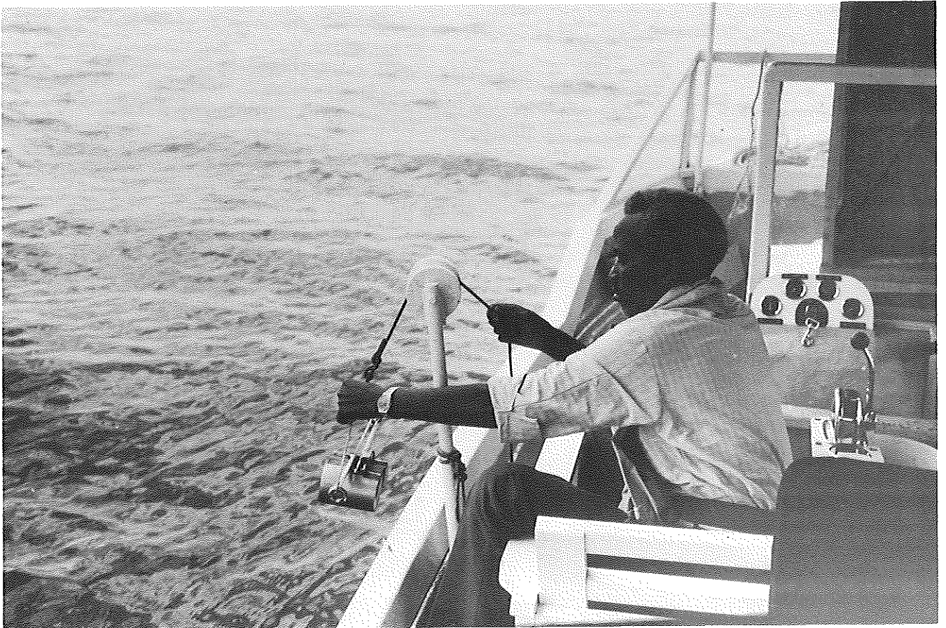
PLATE 9. Collecting a bed sample using a Van Essen grab
