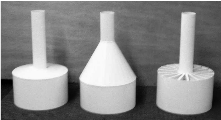
Figure 1: Foundation models used in testing – L-R: concrete-conical-girder
