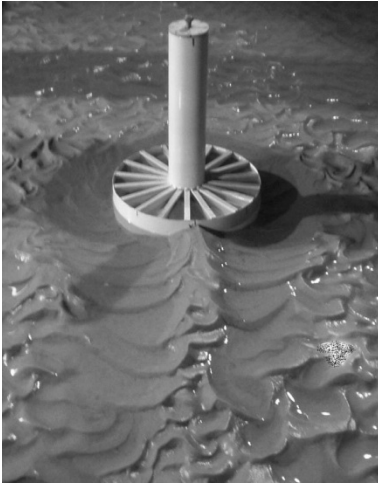
Figure 3: Result of scour test with current (Test 2)
